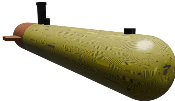
Figure 8.1: Piezoelectric sensitive skin concept.
