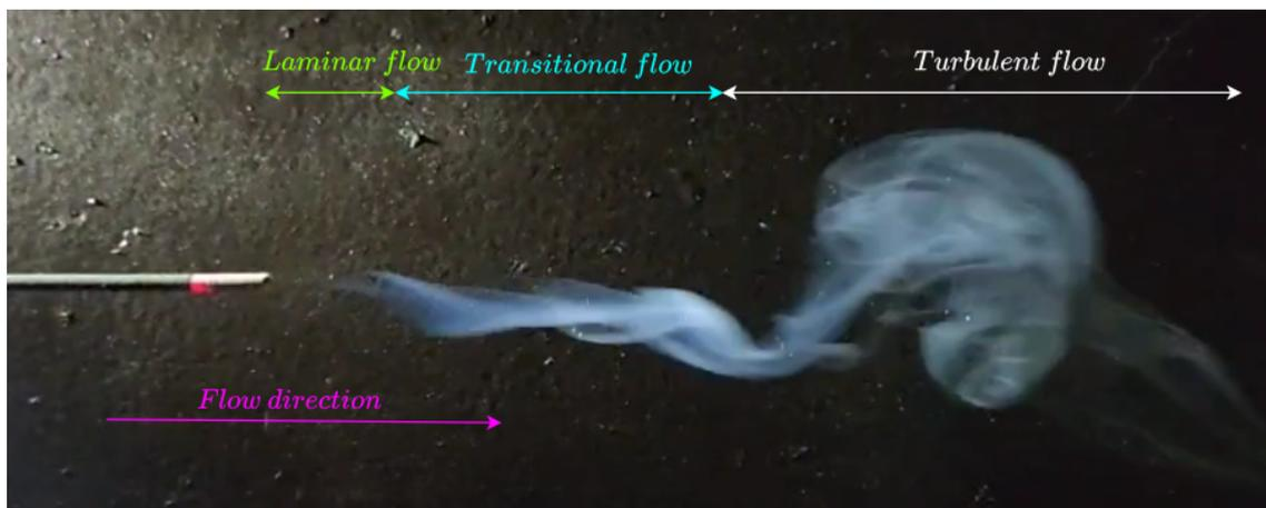
Figure 2.10: Fluid flow transitioning from smooth laminar flow to a turbulent mixed flow.
