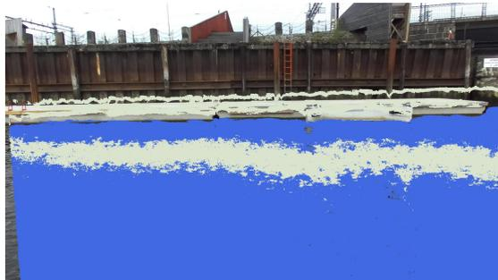
Figure B.1: Multi plane segmentation. Navy blue shows the water plane and the cream color shows the second plane.
