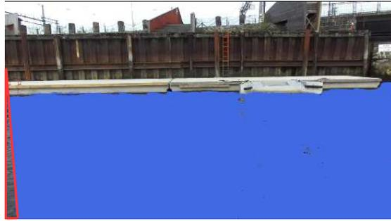
Figure 7.7: Disparity free zone from [RANSAC](#) based plane segmentation
