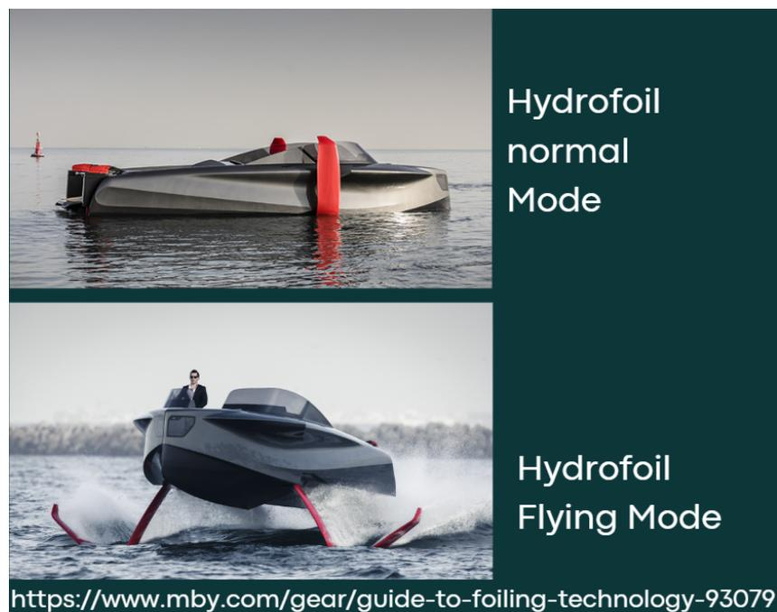
**Figure 3.1:** Two different modes of a hydrofoil. The normal mode is characterized by low-speed/high-drag while the flying is high-speed/low-drag.
