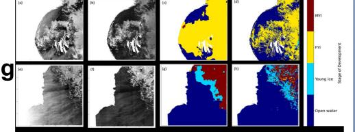
In [4], the author presents a ship-based system for acquiring, processing, and analyzing ice condition imagery using digital images.
