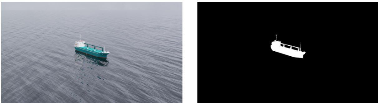
Figure 4.2: Example of an image (left) with the corresponding ground truth mask (right). The quality of the annotation is due to the automatic generation of the ground truth through the simulator.
