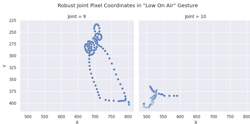
Figure 4.3: Processed pixel coordinates of the left wrist (joint 9) and right wrist (joint 10) keypoints of a diver performing the Low on Air dynamic gesture. The coordinates are less noisy and it's easier to follow motion patterns.
