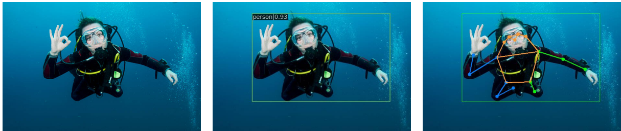
(a) Input image to perform human pose estimation on. (b) Bounding box detected from the input. (c) Pose keypoints estimated with ViTPose.
