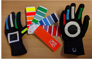
(a) Specialized gloves developed for the CADDY project to facilitate visual detection.
