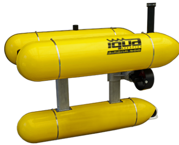
Figure 3.2: Girona500 AUV without attached payload.
