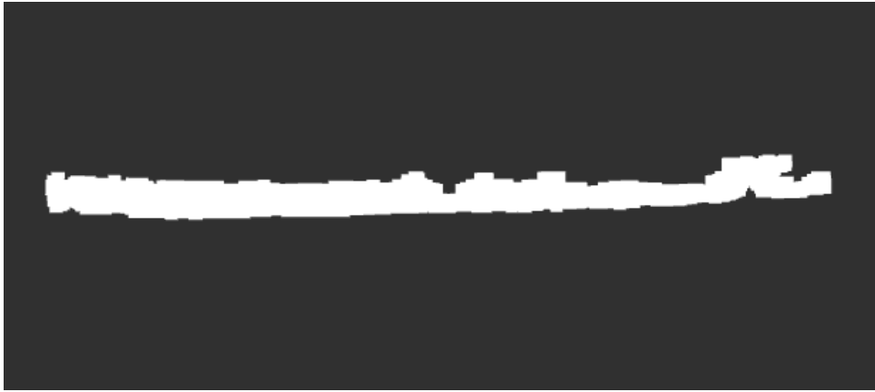
Figure 4.6: Result of color segmentation applied to the underwater scene, showing clear differentiation of the yellow pipe.
