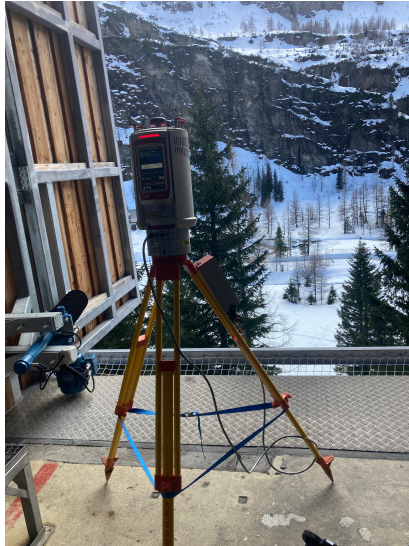
Figure 5.7: Riegl VZ-6000 TLS in the field - Sonnblick Observatory
