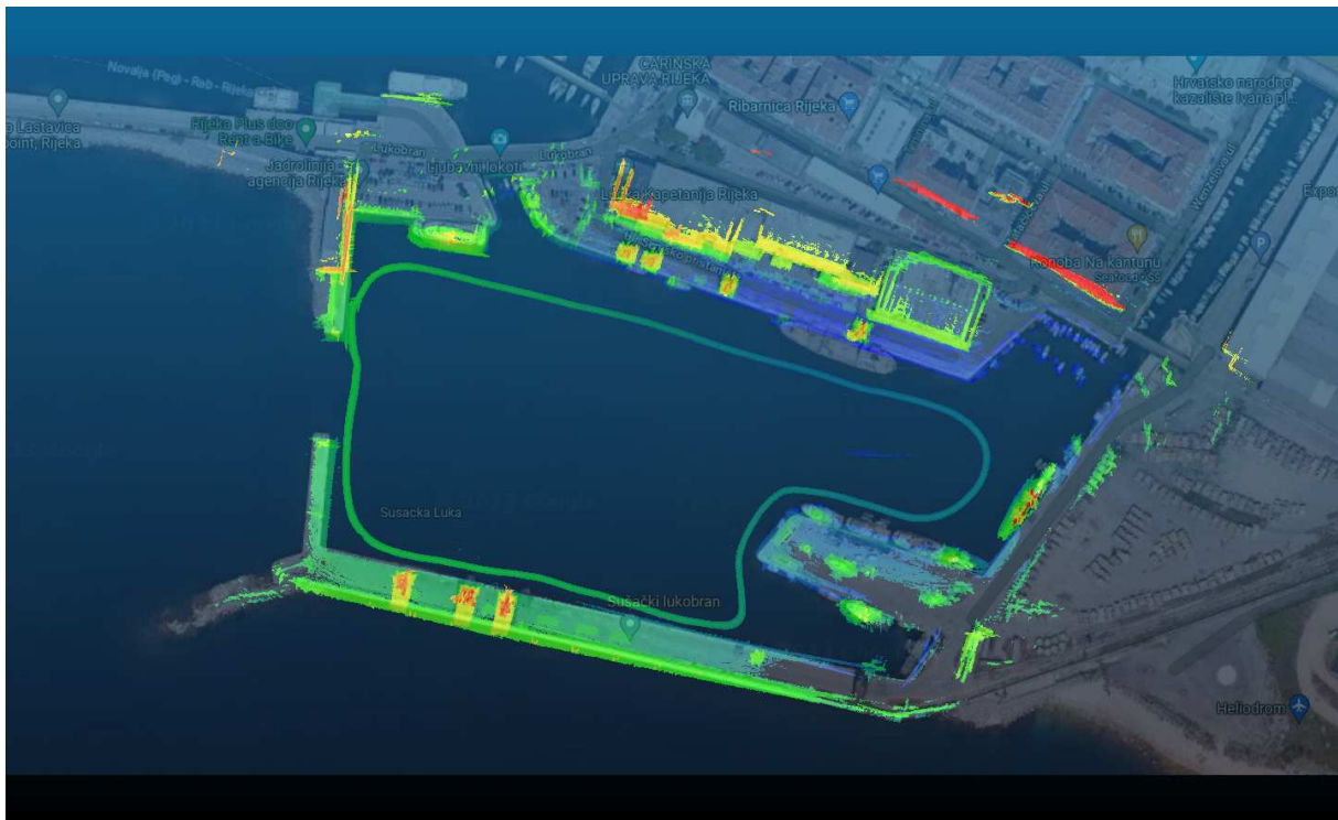
Figure 7.14: 3D SLAM generated map overlaid with Google Maps screenshot - Rijeka Harbour dataset
