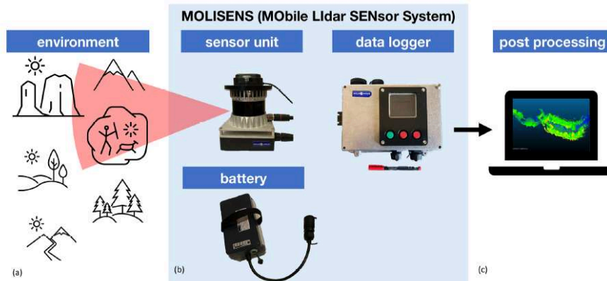
Figure 5.1: MOLISENS hardware components and basic operating principle [5]
