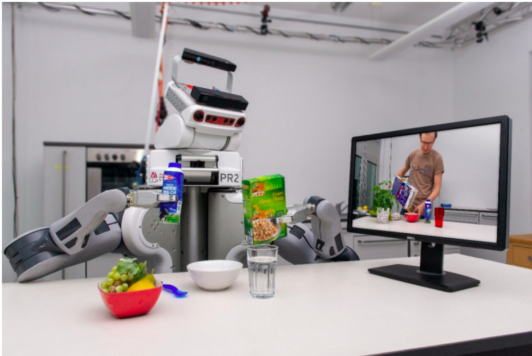
Figure 5.1: PR2 robot learning plans and motions to perform a certain task from a video demonstration.
