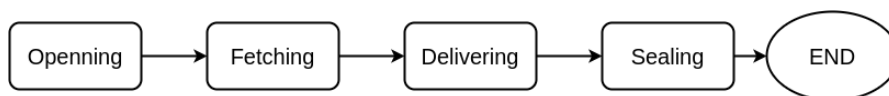
Figure 4.24: Correct task tree that does not loop, this when the model has knowledge of the Top Task, Current Task, and Environment as the model shown in Figure 4.23
