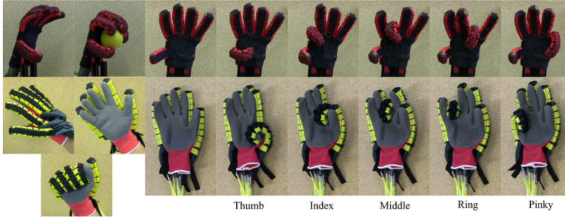
Figure 1.3: Various poses of a soft robotic hand alongside a wearable fabric glove. Source:[10]
